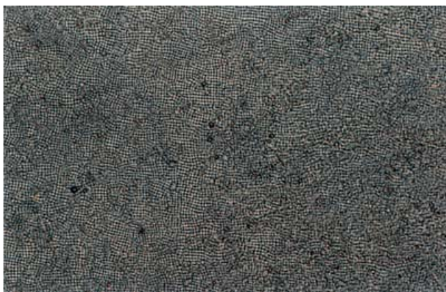
Figure 6. Photomicrograph obtained in the TGB_{C^*} phase at 83^\circ\text{C} while cooling from the SmA phase of the dimer 1g , in planar orientation; note the square grid pattern.
